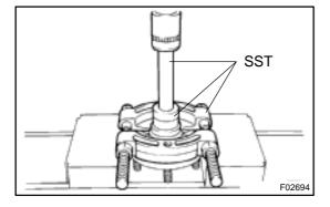
(b) Using SST and a press, remove the inner race (outside) from the axle hub.
