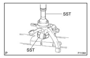
(c) Using SST and a press, remove the bearing. SST 09310–35010, 09527–17011
